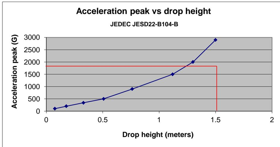
**Figure 2:** JEDEC Acceleration Peak vs. Drop Height
