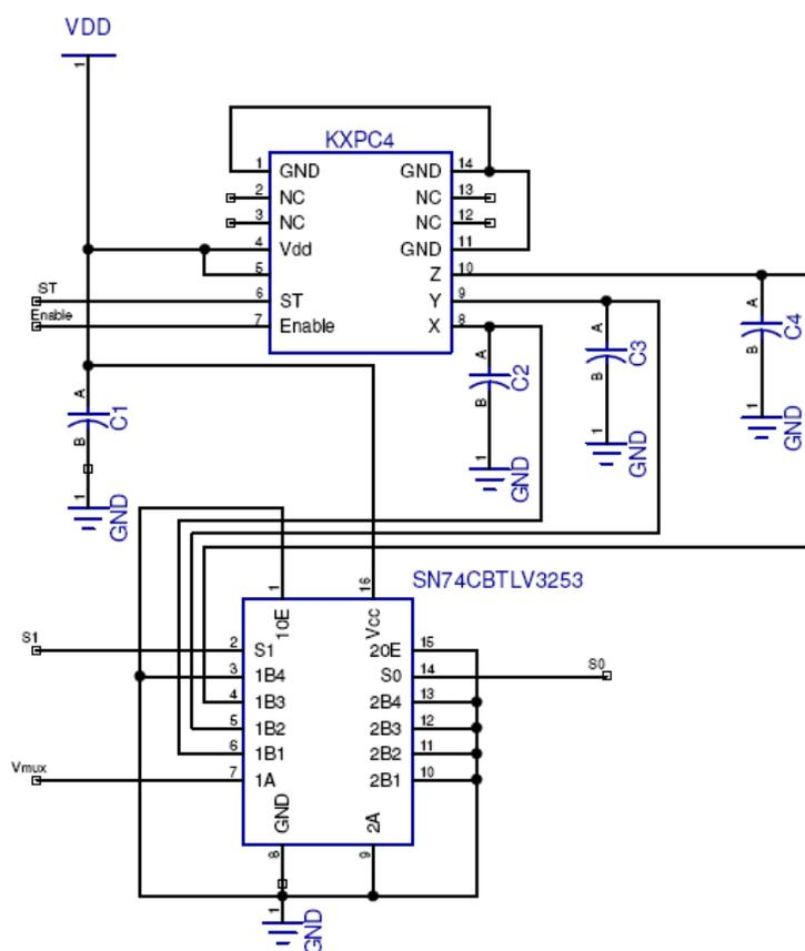
Figure 3: KXPC4/SN74CBTLV3253 Schematic
