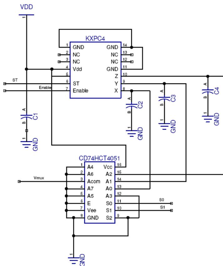
Figure 2. KXPC4/CD74HCT4051 Schematic
