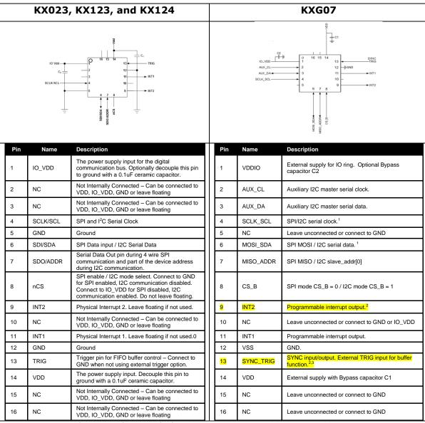
Figure 1: Pin Description KX023, KX123, and KX124 vs. KXG07
