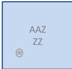
Figure 1. 2x2 mm LGA package marking information
